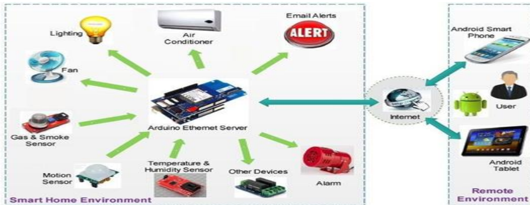
Figure 2: System architecture of the smart home system.
