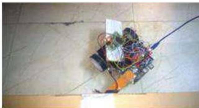
Fig. 22: Ultrasonic sensor detected the wall and robot is giving priority to left direction according to LSRB algorithm
