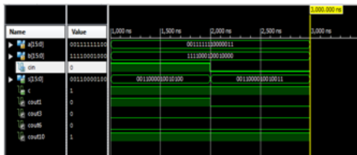
Fig.10: Regular Sqrt CSLA Simulation
