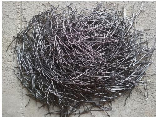
Fig. 2 Mild Steel Hooked End Fibre
