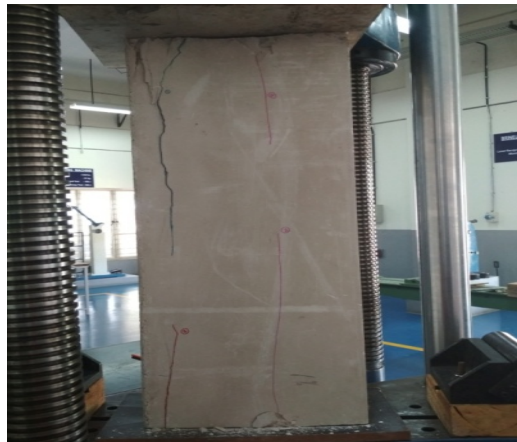
Fig. 4: Failure of column with steel rod
