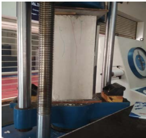
Fig.5: Failure of column with 1.5% SF
