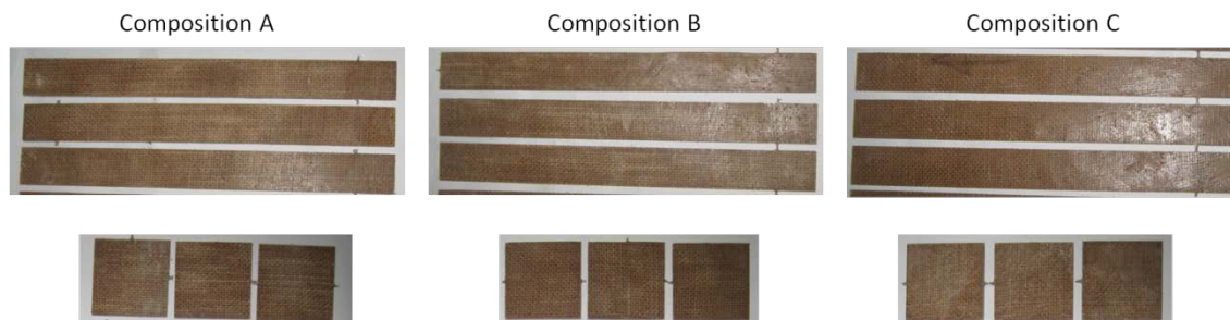
Figure 5: Tension and Compression specimens
