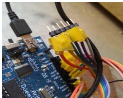
Figure 6: Male connectors at wire ends
