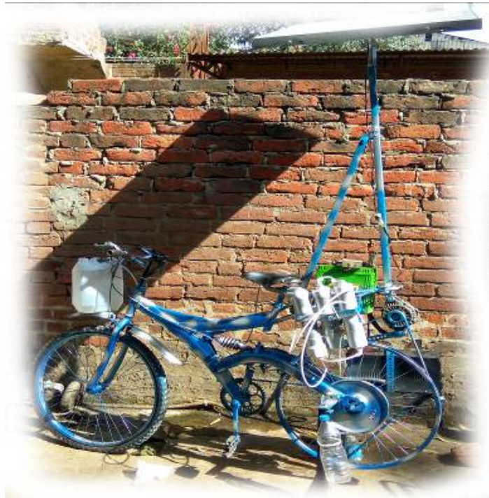
Figure 8: Multistage water purification system
