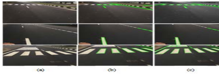
Figure 5: (a) Input Image (b) AHT lane detected Image (c) Fuzzy based HT lane detected Image.
