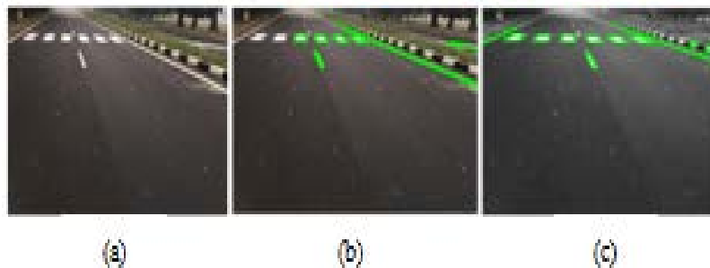
Figure 4: (a) Input Image (b) AHT lane detected Image (c) Fuzzy based HT lane detected Image.
