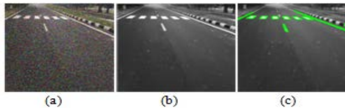
Figure 8: (a) Input Image; (b) JTF Filtered Image; (c) Fuzzy based HT lane detected image with JTF Filter.
