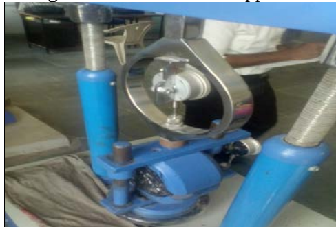
Figure 12: Marshall Test being conducted with the Marshall apparatus
