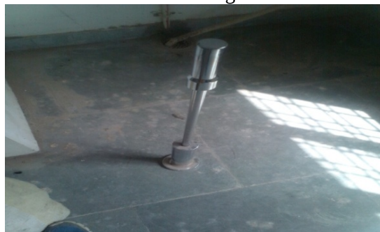
Figure 7: Hammer used for compaction
