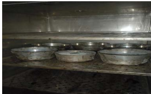
Figure 2: Heating of aggregates and filler mixture in oven
