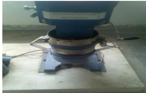
Figure 5: Mixing of aggregates, bitumen, Zeolite and filler
