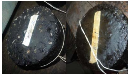
Figure 9: Samples before and after wax coating
